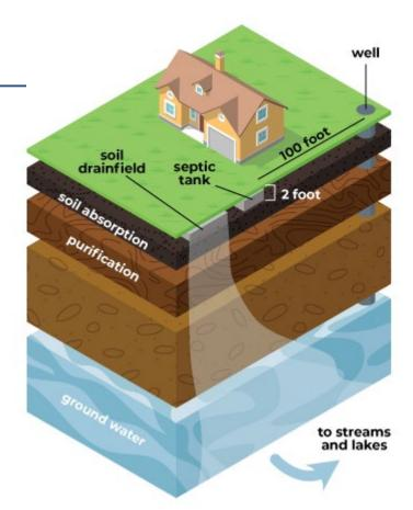
Tank effluent flows to a drainfield where pipes below the surface distribute the wastewater throughout the drainfield. The wastewater then percolates through the soil. As the wastewater moves through the soil, some waste products adsorb to soil particles, while microorganisms in the soil ingest other waste products, providing final treatment of the wastewater.
